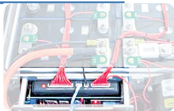
Case 1: Old battery home equalizer is implementedDynamic equilibrium changes to active equilibrium
